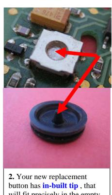
will fit precisely in the empty space left after removal of the plastic knob
