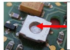
Due to ageing, plastic knob became brittle, deteriorated and detached from the top of electronic switch.
