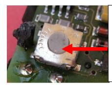
Plastic knob is still attached but shows signs of deterioration.
