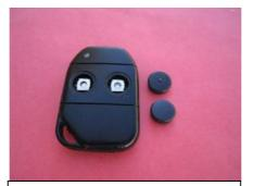
**5.** Once switches are clean and shell is free of old rubber buttons, you are ready for button replacement.
