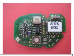
**3.** Open remote on the split line and separate electronic part from hard shell top part. Remove old rubber insert and any remnants of the old rubber key buttons from the shell. You can use small flat screw driver.
