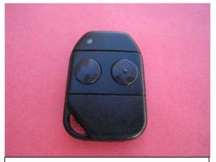
**7.** Next press new buttons in and put your remote together in reverse order. Once buttons are inserted, your remote is ready for use as no re-programming is needed.
