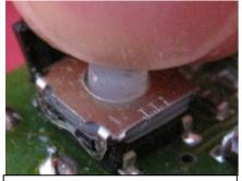
**4.** Next remove deteriorating plastic knobs from the top of switches. Simply scrape them off using your finger nail.
